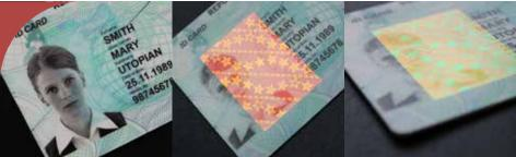
Opalux's Polycarbonate ID-Lock is highly transparent at most angles (left). At select angles, PC ID-Lock's vibrant, multi-colour colour-shifting reflections catch the eye (centre) and colour-shift (right). This optical variability permits PC ID-Lock to protect personalised information in polycarbonate documents, without interfering with document legibility.
